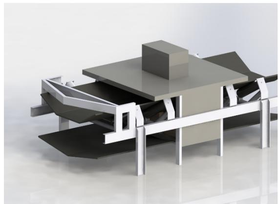
Equipped with high-tech gamma detectors and high-performance electronics, the online cross-belt analyzer has technical characteristics for accurate measurement of elemental composition of raw mixtures and bulk materials. Due to this, the elemental analyzer can be used in a range of applications such as sorting, blending, raw mix control etc. In addition, our smart algorithm automatically adapts to changes in the composition of the mixture or material on the belt.
